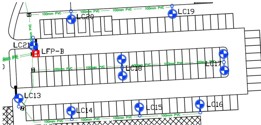
Figure 9: Typical car park lighting layout using 8m high single and twin-arm columns
